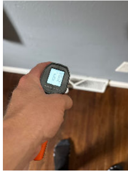
Cool Air Temperature First Floor.
