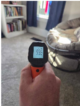
Warm Air Temperature Second Floor.
